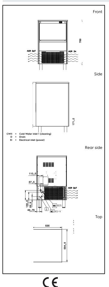
Supply voltage: 220-240 V/1N ph/50 Hz Electrical power, max: 0.37 kW Capacity: Bin capacity: 25 kg Key Information: External dimensions, Width: 535 mm 595 mm External dimensions, Depth: External dimensions, Height: 894 mm Net weight: 56 kg Output: 56 kg/day Kind of cube: Ice Cube 40 g **Sustainability** R290 **Refrigerant type:** Refrigerant weight: 65 g Water consumption: 30.5 lt/hr
